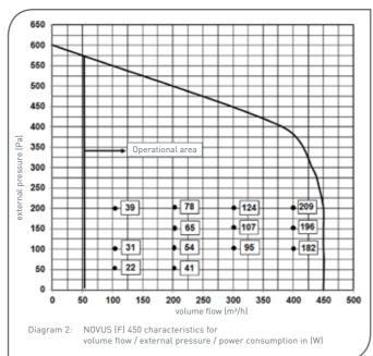
Note: the figured number values in the diagram of the p-V-characteristic curve give the power consumption in [W] in the corresponding operating points and are valid for NOVUS 300 (diagram 1) or NOVUS 450 (diagram 2) respectively with standard heat exchanger without integrated defroster.
